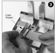
When installing a plug on the end of a cable, use the cable stopper to correctly position the cable.
