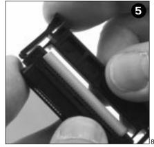
The 101XX-8000 plug may be assembled with a strain relief that is installed on the topside of the plug. Bend cable over the top of the connector and snap both inside and outside latches into the body.
